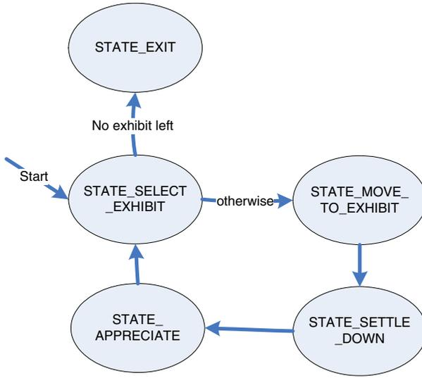
**Fig. 3.** Finite state machine controls visitor behavior
