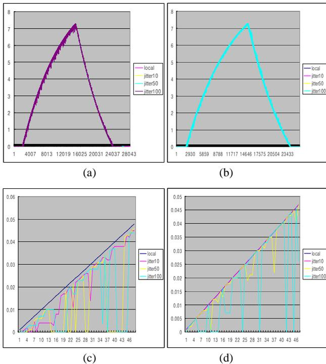
**Figure 10.** Force feedback according to various jitters: (a) Position Transfer Model, (b) Force Transfer Model, and (c) Magnified view of Position Transfer Model around the beginning point (d) Magnified view of Force Transfer Model around the beginning point
