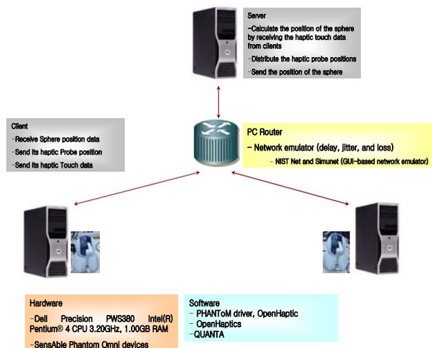
Figure 4. Hardware setup for haptic collaboration test bed
