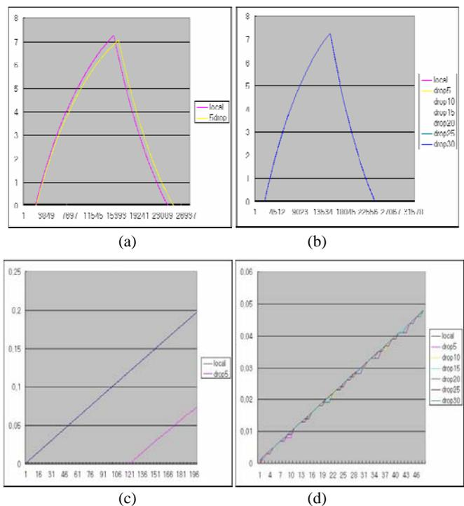
**Figure 8.** Force feedback according to various losses: (a) Position Transfer Model, (b) Force Transfer Model, and (c) Magnified view of Position Transfer Model around the beginning point (d) Magnified view of Force Transfer Model around the beginning point
