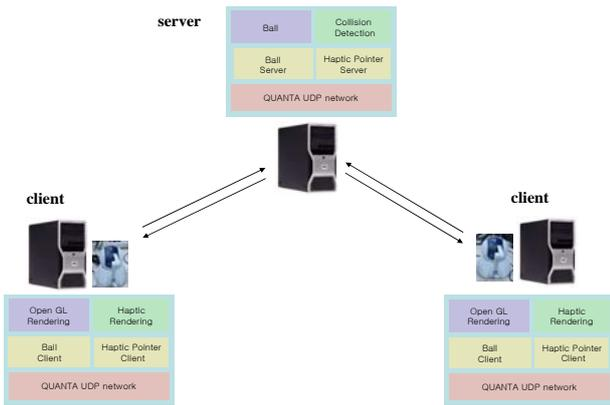
**Figure 5.** Software architecture of experimental haptic collaborative system
