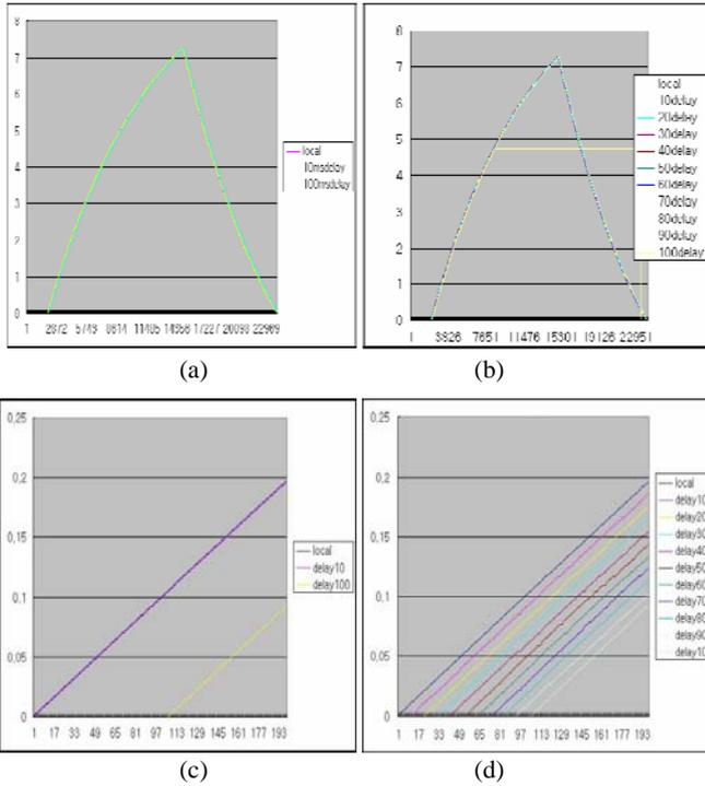
**Figure 9.** Force feedback according to various delays: (a) Position Transfer Model, (b) Force Transfer Model, and (c) Magnified view of Position Transfer Model around the beginning point (d) Magnified view of Force Transfer Model around the beginning point
