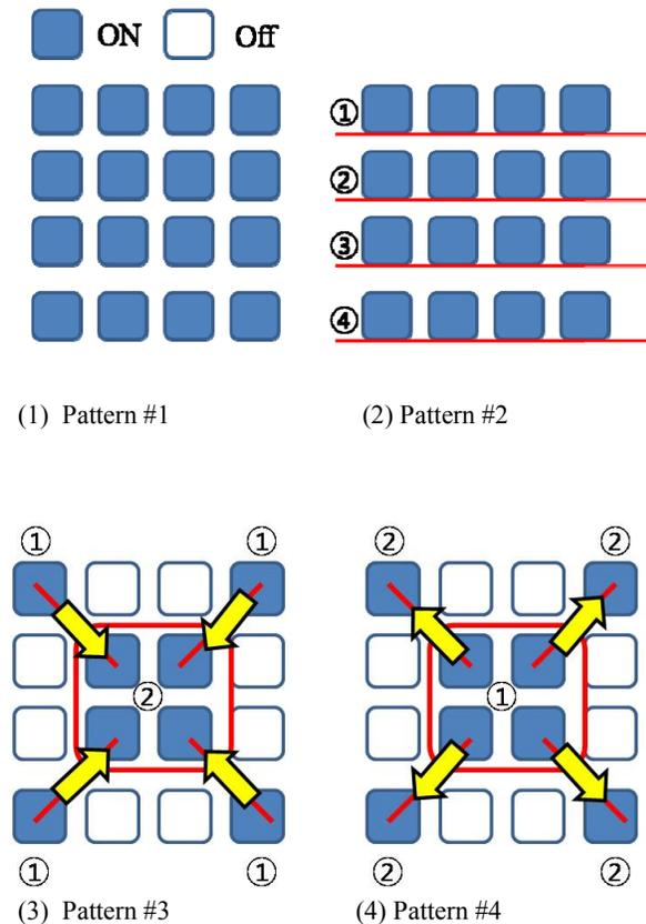
Fig. 7. Examples of Different Vibrations Patterns
